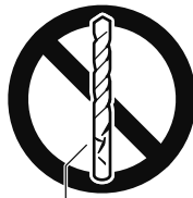
Shank section Scratches, dents, etc.
