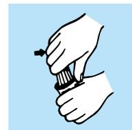
While holding the HDC nut firmly in one hand grasp the FDC collet in the other while pushing sideways.
