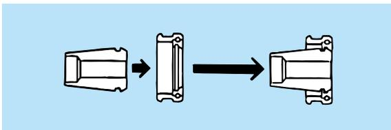
Place the FDC collet into the threaded end of the HDC nut. Press down on the rear of the collet to "clip" the collet into the nut.
